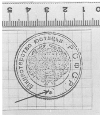
FIG. 9—The random points were made by excess metal points on the cachet. 1 in. = 25.4 mm.
